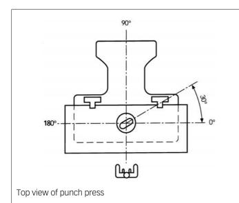
**Attention:** in case of order please specify the position of the references placed on the die housing of the machine (not only the shape orientation respect the die).
