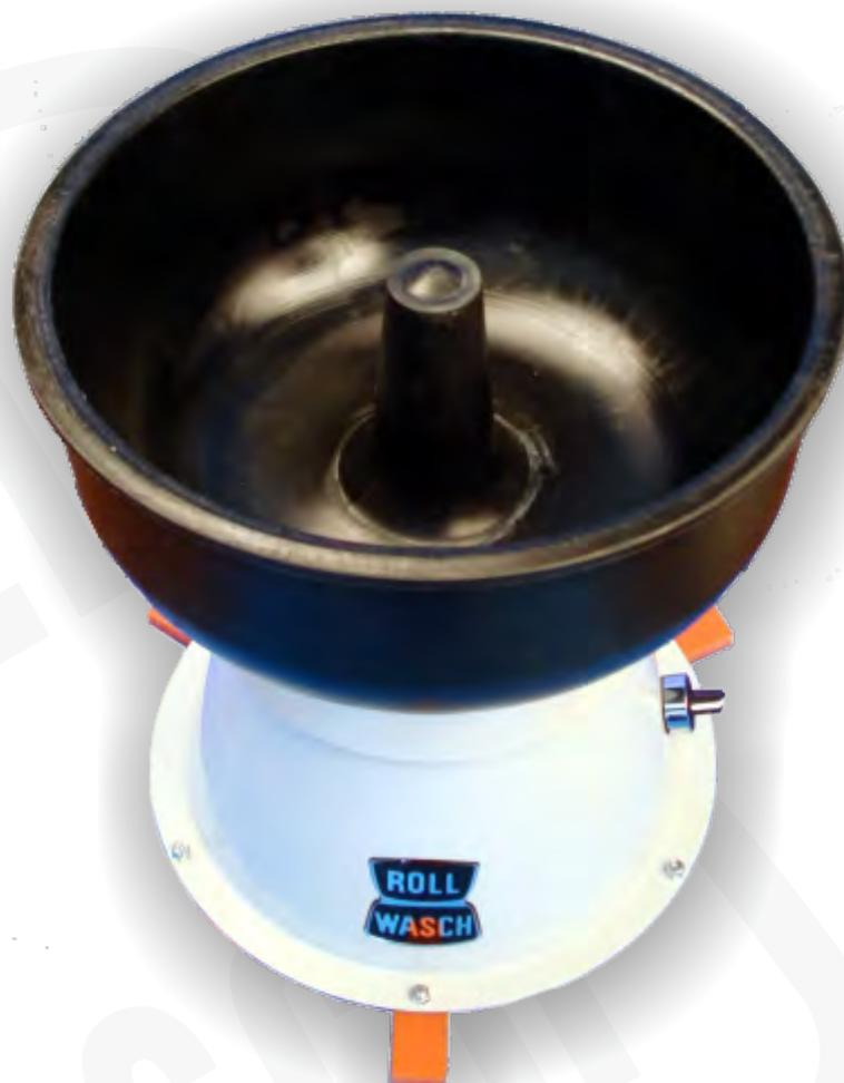
A series of professional vibratory machines, with a monobloc motorvibrator made in aluminium with eccentrics adjustment, a polyurethane tank as the industrial machines and strong design. Functional and handy, MINOR-XS can run both dry and wet cycles, thanks to a removable draining filter that can be replaced with a polyurethane cap. Ideal for the finishing of small pieces, small batches, laboratories, hobby.
